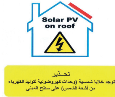
Figure 8 – Sign to be used to indicate the presence of a PV plant
