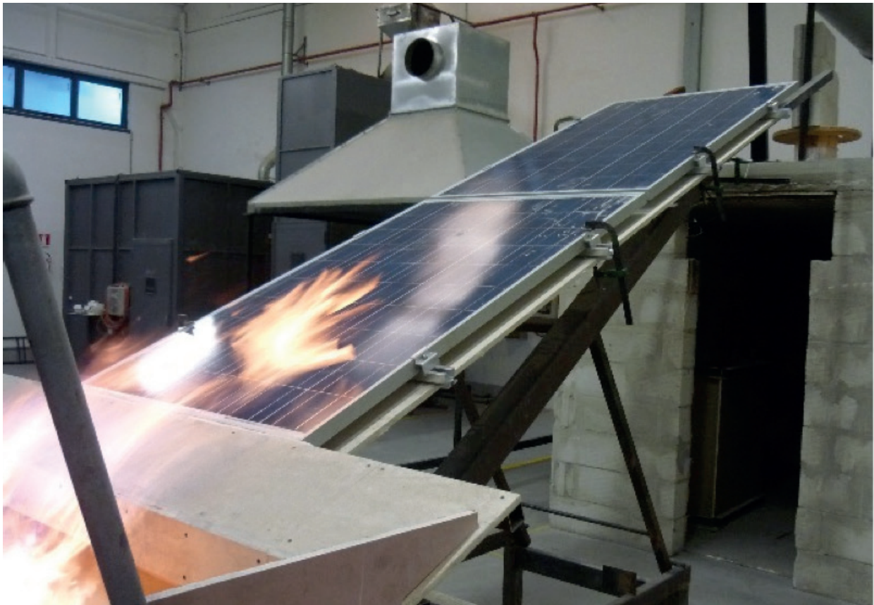
Figure 1 – Spread-of-flame test (LAPI laboratory)
